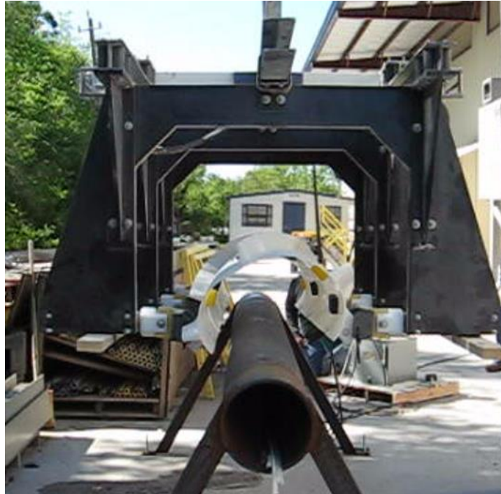
ROV strake installation tool installing strake onto pipe
