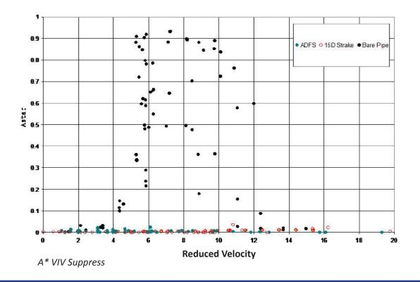
A\* vs. Reduced Velocity show the A\* and the Cd (Drag Coefficient) of both the ADFS and the AIMS Strakes.
